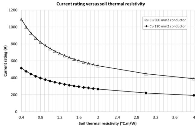
Fig. 8, Current rating vs native soil thermal resistivity.
