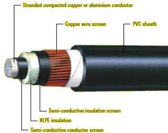
**Fig. 13, Cross-sectional view of 11 kV cable modelled.**
