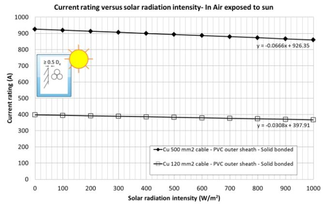
**Fig. 3, Current rating of 120 mm<sup>2</sup> and 500 mm<sup>2</sup> cables exposed to varying solar radiation intensity.**
