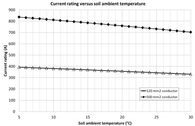
**Fig. 11, Current rating vs soil ambient temperature.**
