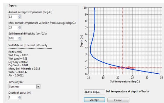
**Fig. 12, Calculation of soil ambient temperature at a particular depth and time of year.**
