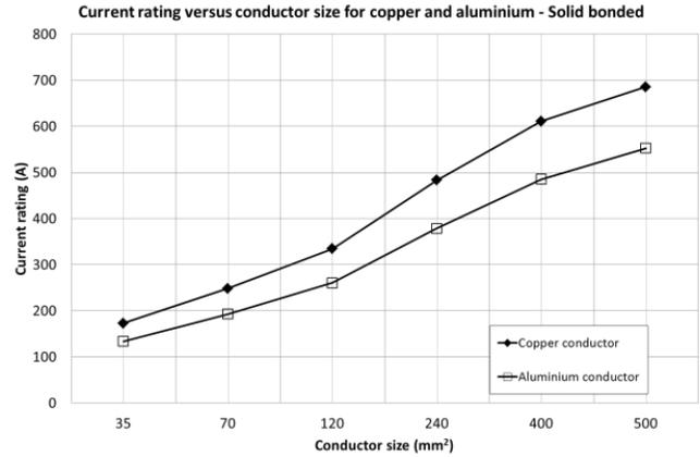
Fig. 7, Current rating vs conductor size for copper and aluminium conductors – cables direct buried.
