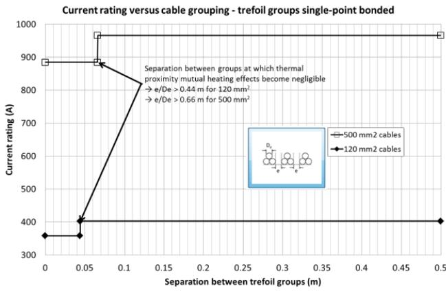
Fig. 5, Current rating vs separation between trefoil groups.
